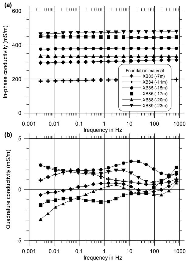
Figure 2. *Complex conductivity spectra of material from dike foundation. The samples are taken from the borehole at km 138.358. (a) In- phase conductivity. (b) Quadrature conductivity.*
