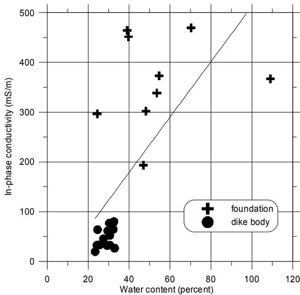
Figure 4. Relation between water content and in-phase conductivity at 2.9 Hz.
